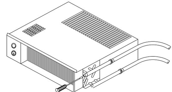
4. Isolate electrical supply and connect the transformer flying leads to the fused spur (3A). The transformer must be located outside the bathroom or high humidity area. Connect the single-pin male connectors to the twin core cable you have supplied.
