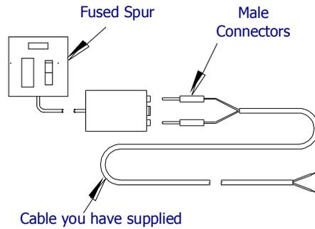
5. Push in the connectors to the transformer terminals and connect the other end of the cable to the terminals on the back of the product.
