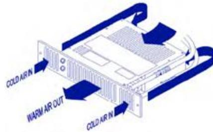
Space Saver includes an internal thermostat that prevents the fan from operating until the central heating system water passing through the heat exchanger reaches 38° C. This prevents the Space Saver circulating cooler air at start up.
