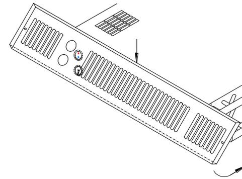
7a. Fit supplied grille over top flange, locate over switches then press lower edge backwards, as shown in diagram, to fix grille in place.
